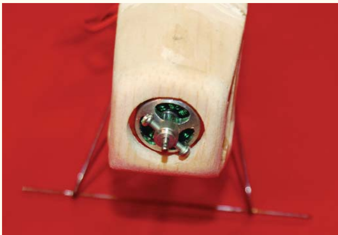
The CustomCDR Baby Bullet (Cool Wind) brushless motor weighs just 16 grams and has a thrust output of approximately 12 ounces.
