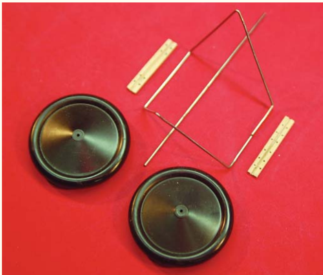
The landing-gear structure is fabricated from two pieces of .047 ( \frac{3}{64} inch) music wire. Guillow's 2-inch lightweight plastic wheels are used.
