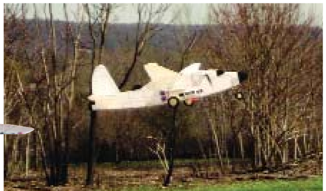
The B-26 climbs out just after liftoff. Notice how the foam-board wings bend slightly under the load, giving extra dihedral angle.
