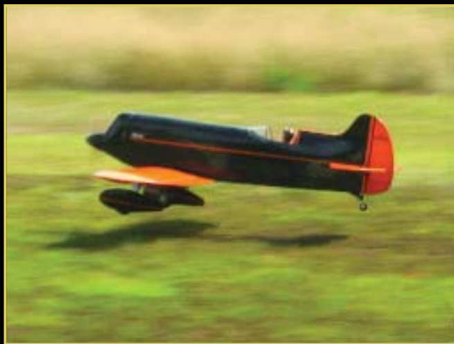
After a full-power run of roughly 50 feet, the model lifts off smoothly. The wide-track gear absorbs many of the bumps in the grass.
