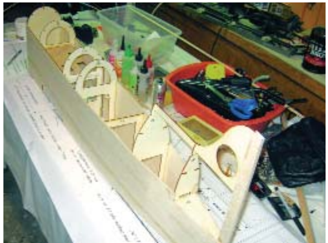
Bevel the tail post and then glue it in place. Dry-fit the fin and the remaining formers to assure good alignment.
