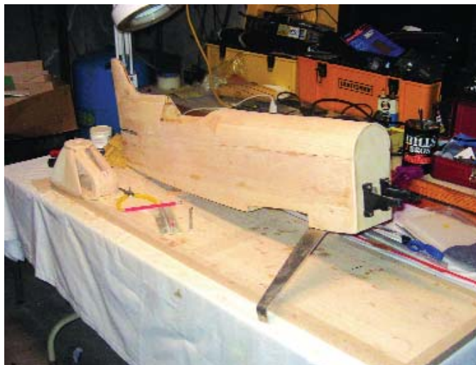
Once the sheeting is complete, it's a good time to test-fit the landing gear and engine mount. The cockpit area can be detailed at this time.
