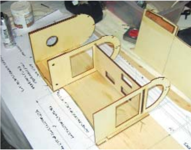
Formers F1 and F2 have been put in place, and the servo plate has been mounted between them.
