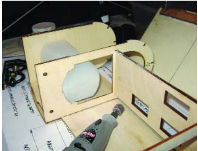
With the fuselage wide open, it's a good time to fit the fuel tank. Silicone sealant will be used to mount the tank permanently.
