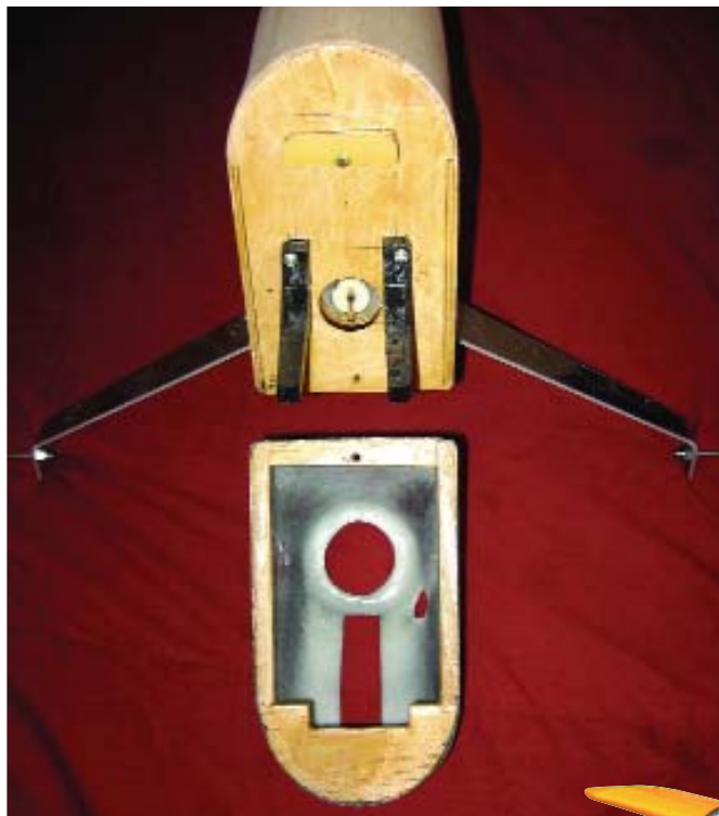
Once the sheeting is complete, it's a good time to test-fit the landing gear and engine mount. The cockpit area can be detailed at this time.
