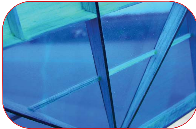
The carbon-fiber capstrips give the high-aspect-ratio wing its required strength. Those capstrips run full chord on the bottom of the wing but only halfway down on the top of the wing.
