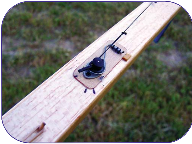
Texas Timers' button-type viscous timer is set up using Gene Smith's "mousetrap" arrangement to take direct pressure off the timer. The marks denote the length of timer runs.
