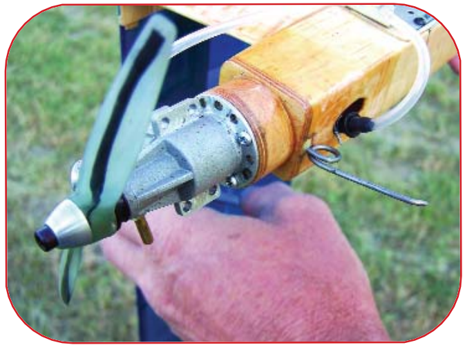
The pressure tank tucks up into an opening in the bottom cross-grained sheeting just aft of the firewall. The propeller is carbon-reinforced fiberglass, to handle the high-rpm loads.
