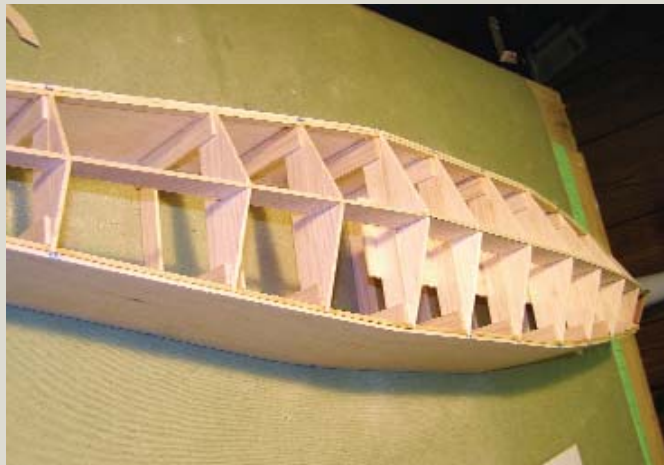
The fuselage is built upside down. The balsa floor is glued in place at this stage. It will be used later as a place to locate the power-system batteries.
