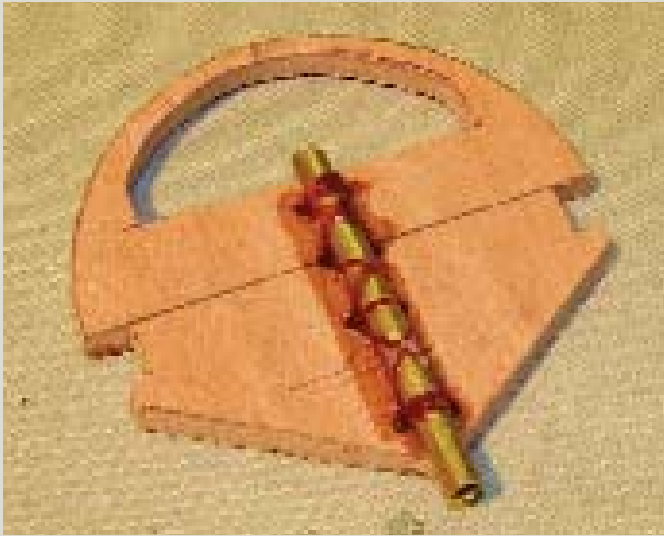
Former FI has \frac{5}{32} -inch-inside-diameter brass tube attached to it for holding the nose-gear leg. The Kevlar thread is saturated with epoxy resin after alignment is confirmed.
