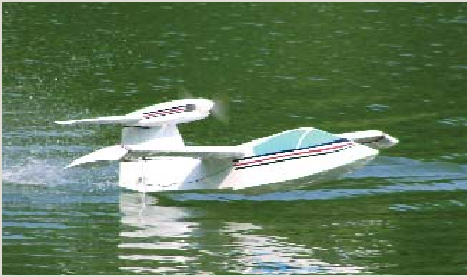
The Spectra II can be slowed to a crawl for landing in tight spaces. The position of the elevator relative to the propeller aids in performance.
