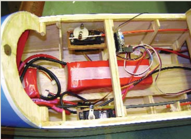
The forward hatch secures the two 3S batteries wired in series. The servos shown operate the rudder and elevator control. Note the magnetic closure.
