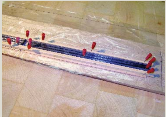
Make the wing joiner by gluing three carbon-fiber tubes together. Thick cyanoacrylate is recommended for construction because it bonds extremely well with the composite material.
