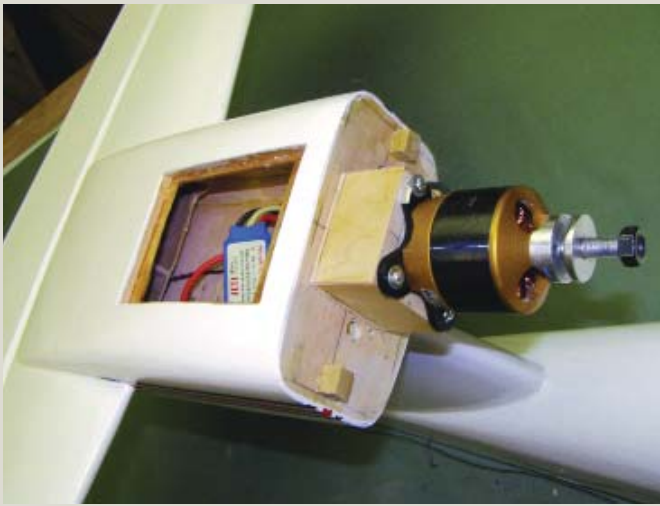
The Spectra II is convertible from electric to glow power. An AXi 4120/18 with a Jeti 70 opto ESC does the job of a .46-size engine when powered with a 6S Li-Poly battery system.
