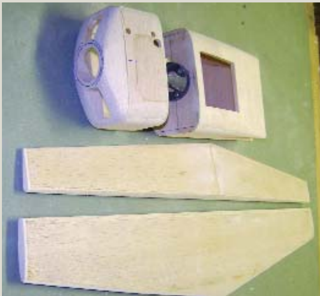
Below: The nacelle and tail surfaces are finish-sanded and ready for final assembly. Now is a good time to get the hinging finished.
