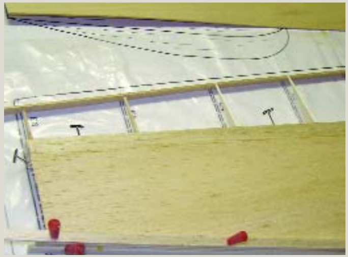
The stabilizer sheeting joins the high edge of the full-length balsa spar. Build the stabilizer in right and left sections, and join them after the sheeting is complete.
