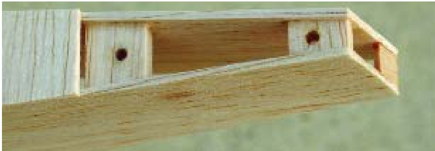
Stabilizer mounting blocks are inset \frac{1}{16} inch from the bottom of the fuselage sides to provide clearance for the stabilizer doubler. Mounting holes have been tapped for 4-40 nylon screws, which attach the stabilizer.
