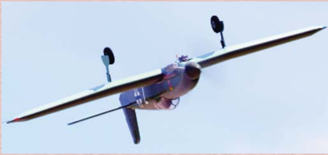
The inverted gull-shape wing is pronounced just enough to enhance the scale appearance. Flap sizes and deflection ratios were carefully considered.
