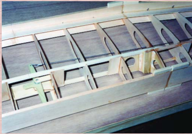
Adding 5/16-inch "feet" on the top and bottom of each end of the fixture pieces makes it possible to use less than straight wood without introducing stresses when attempting to straighten it.
