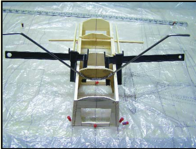
The piano-wire landing gear is stitched to the former with thread, Kevlar, or copper wire. The lower wing's center-section is built into the forward framework.
