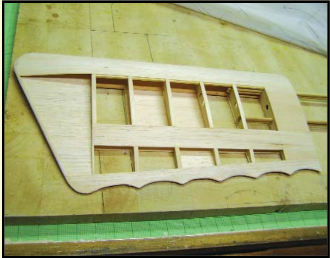
The wide sheeting near the TE is centered over the hinge line. Once the aileron is cut away, cap the open areas with balsa.
