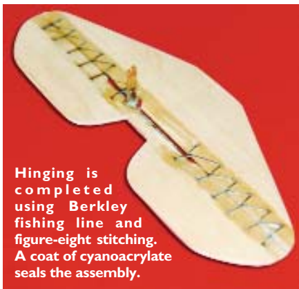
As are the fuselage and wings, the horizontal tail components are made from basswood sheets. All surfaces should be smoothly contoured.
