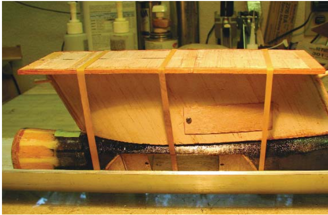
A small box to house the Walston radio transmitter is installed in the left side of the pylon; an exit tube runs from the box out the rear.
