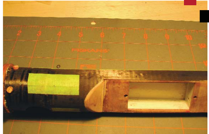
Sand the fuselage smooth prior to any installation. The engine assembly is aligned with quadrant marks and pinned with dowel rods epoxied into several points.
