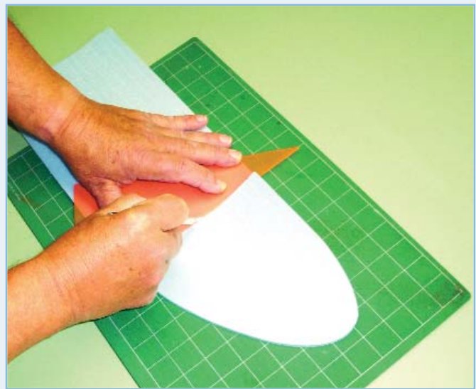
Separate the wingtip from the polyhedral joint location. This is a good time to paint the bottom of the tips a bright color.
