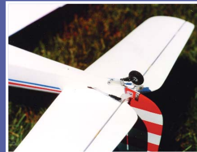
The author used Klett hardware throughout. Pushrods from the forward-mounted servos should be hard wire, to prevent trim changes caused by temperature.
