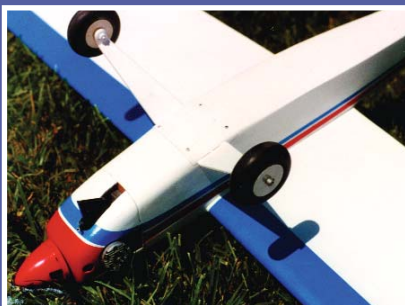
A balsa hatch covers the landing gear and is held in place with 4-40 bolts and blind nuts. Several landing-gear types can be used.
