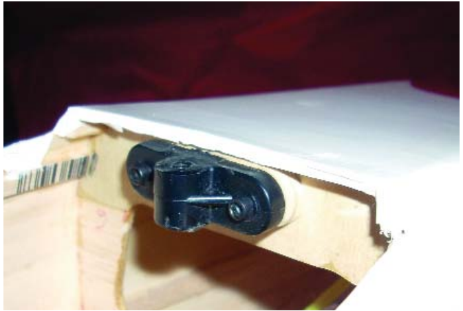
The wing mounting bracket is shimmed to sit forward of bulkhead #6 and approximately 1/4 inch below the fuselage skin. It is tapped with 10-28 threads.
