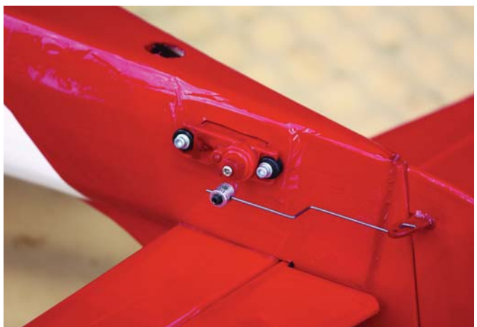
The MPX-50 servos have been painted with matching Testors enamel, which makes them almost invisible. Plans show custom control horn templates.
