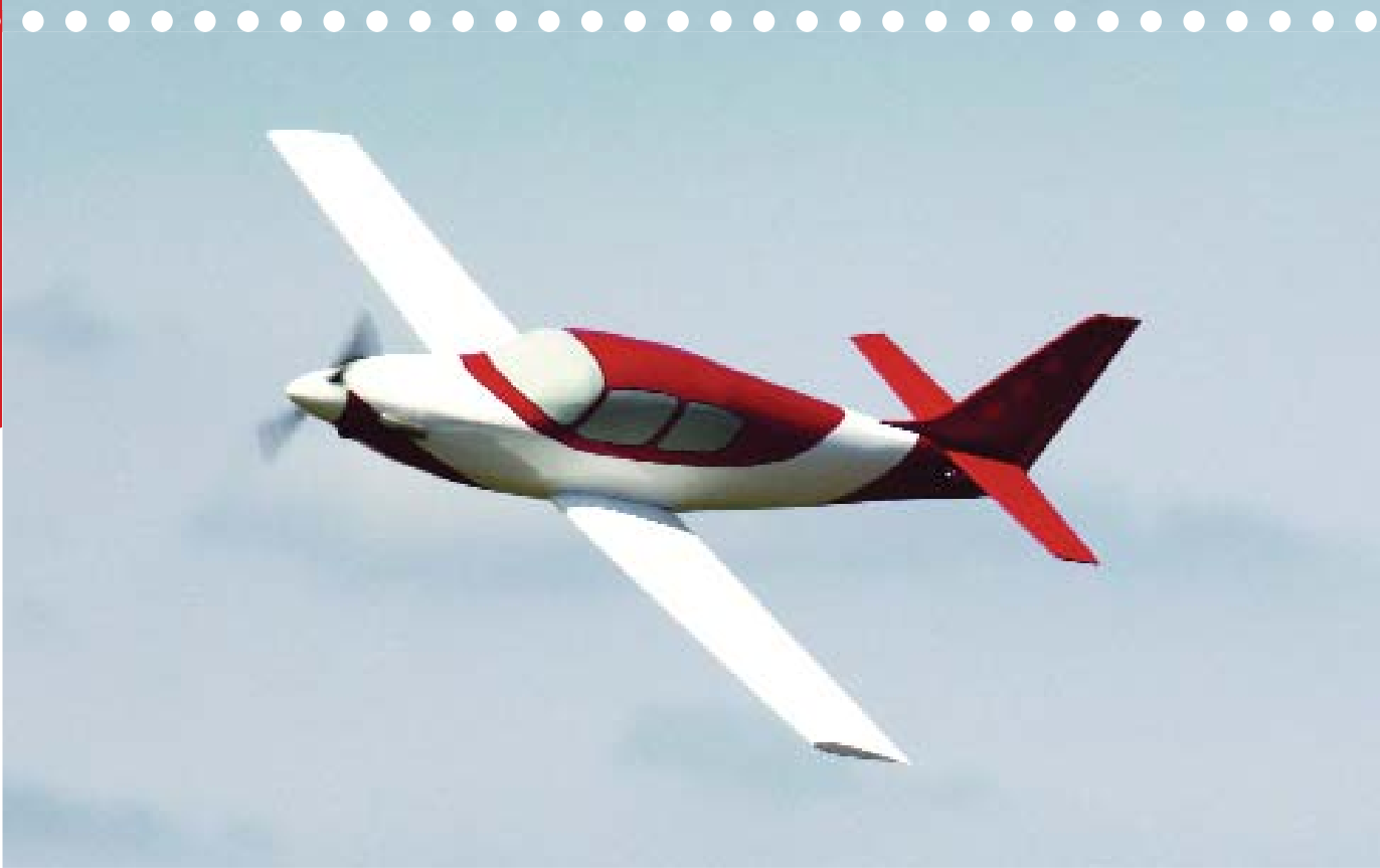
The Lancair will cruise at roughly three-quarters throttle when equipped with a Cobalt 400 motor and eight-cell NiMH batteries. Stall characteristics are predictable. Smith photo.
