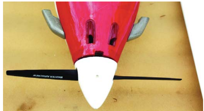
Ram air, through Heyes hooded pushrod covers, provides cooling for the motor and electronics. Exhaust pipes are carved from balsa and painted.
