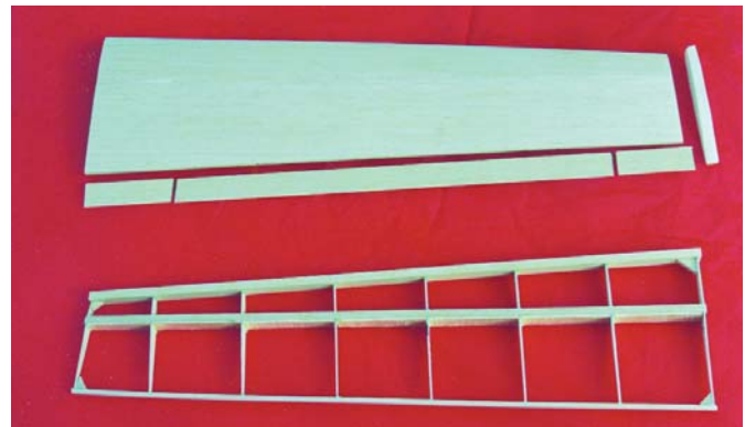
Wings are skinned with 1/32 balsa sheet after removal from the building board, and then TE components are added. Corner braces firm up the joints.
