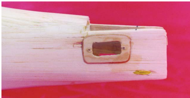
Elevator and rudder servos (9 grams each) mount in the tail, inside plywood frames that are surface-mounted to the fuselage balsa skin.
