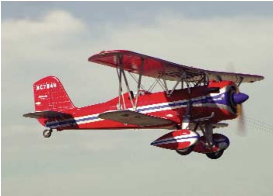
The 4E is flown on 0.018-inch-diameter, 52½-foot-long braided-cable lines. It's a good configuration for CL, and the model's wheel placement guarantees good ground handling. Ramsey photo.
