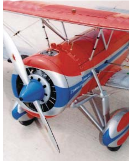
The 4E is flown on 0.018-inch-diameter, 52½-foot-long braided-cable lines. It's a good configuration for CL, and the model's wheel placement guarantees good ground handling. Ramsey photo.
