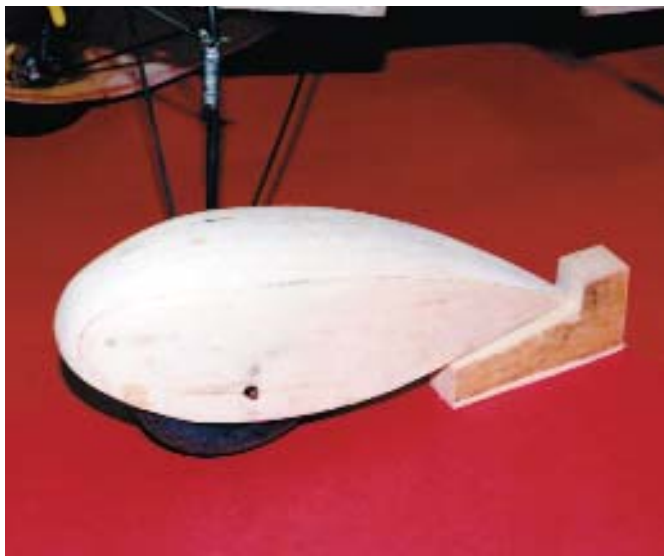
A 1-inch-thick balsa block is used to precisely locate and line up the wheel pants. Locate and epoxy one pant in position. Transfer the block to the other and secure the second wheel pant.
