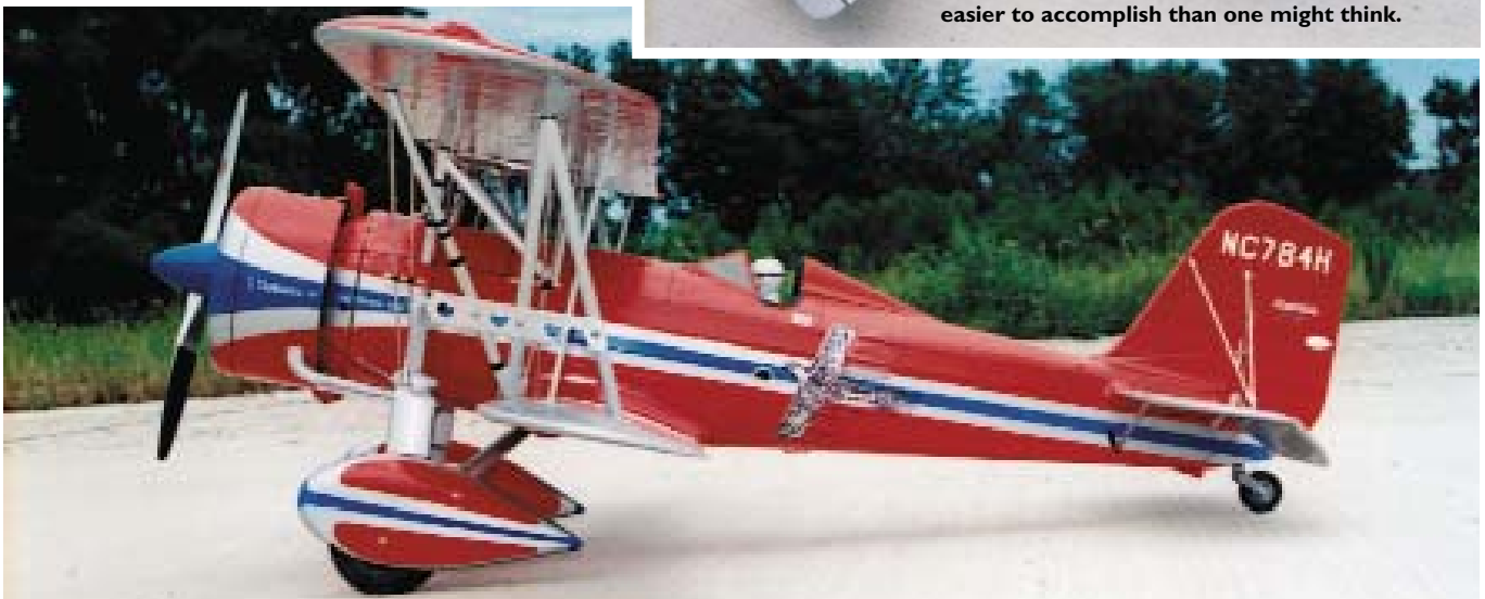
Frank's Stearman is a typical counterclockwise setup with the leadouts on the port side. An O.S. .46 two-stroke engine is more than enough power.
