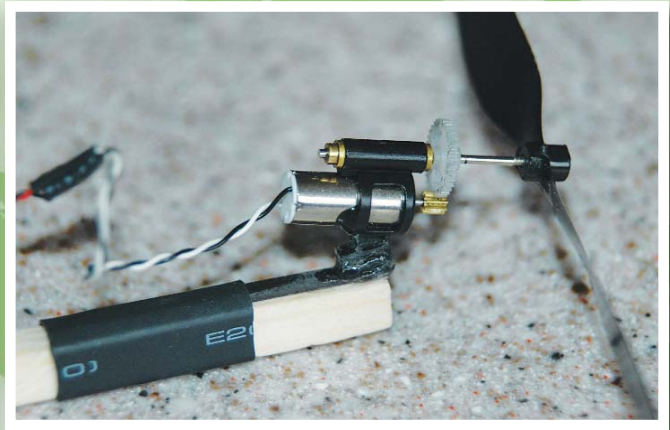
A ParkZone Ember motor system powers the 100% version. The downthrust shown might not be everyone's taste, so feel free to take some out.
