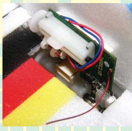
Servo tape is also used to attach the Spektrum AR6400 control module to the fuselage. Locations on the plans assure that the stock radio wiring works without extensions.
