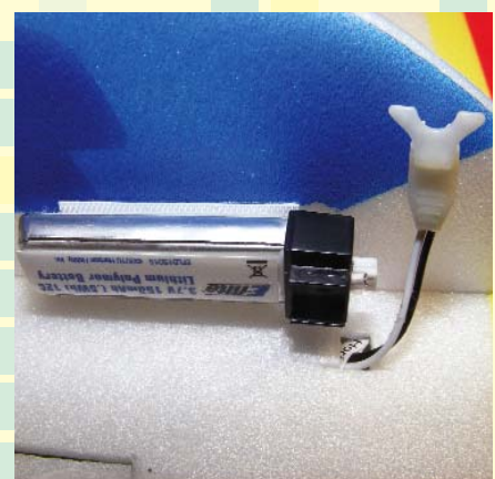
Once the proper CG is located, attach the single-cell, 150 mAh battery in place with the included hook-and-loop material.
