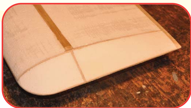
The wingtip has its foam blocks glued in place on the balsa parts and has been shaped with a sanding block. The bare foam wing cores are covered with a low-temperature iron-on film.
