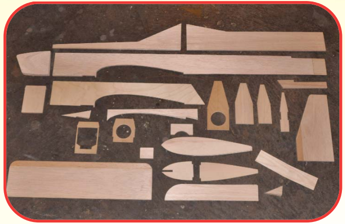
This is the rest of the balsa and plywood parts that need cut out for the fuselage and tail surfaces. All together, it's a short list of kit components.
