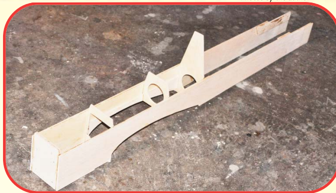
The basic fuselage structure begins with balsa sides and plywood doublers, joined by the first four plywood bulkheads. The next job is to pull the tail together straight.
