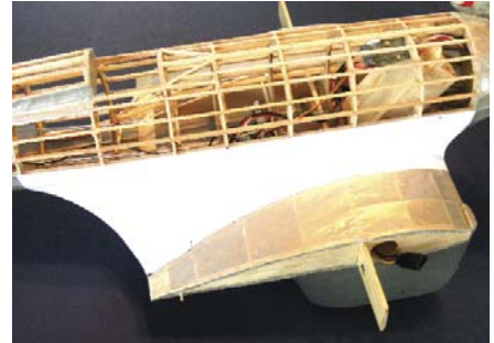
A partially completed frame sits on the bench amid construction clutter. The Gamma is starting to take shape! The completed model should weigh slightly more than 16 ounces.
