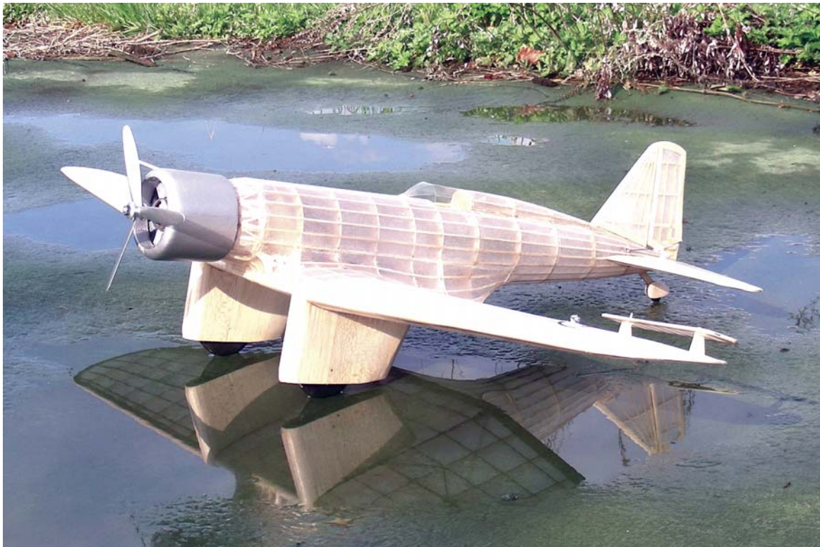
The prototype model was covered with nonsilvered Japanese tissue and then painted with a light coat of Krylon silver and trimmed as the Texaco racer. Silver dope could have been used and would have been somewhat lighter, but the airplane has a good margin of performance.
