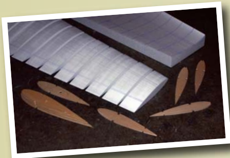
The balsa ribs match the foam patterns. They will fit perfectly into the fixture for wing assembly. The way this works is brilliant!
