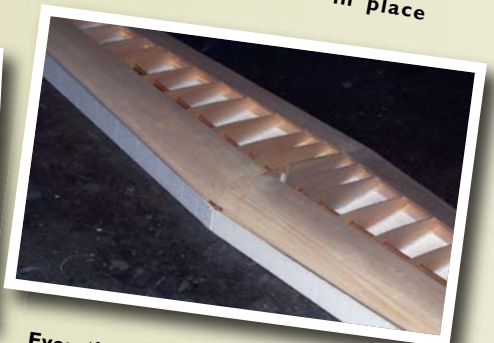
Even the dihedral angle can be cut into the foam building fixtures, so that the wing panels can be tightly and easily joined.
