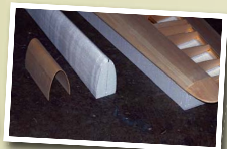
A short test piece of balsa sheeting has been formed to illustrate the function of the process. The LE sheeting will fit perfectly in place over the wing ribs.
