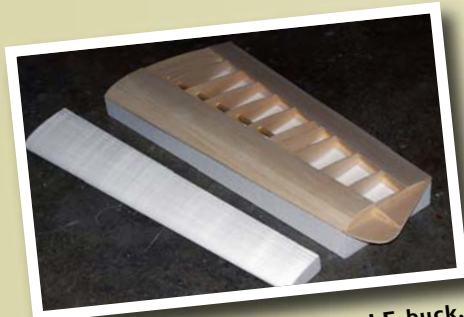
The loose foam piece is the LE buck, made to form the LE sheeting. The sheeting is soaked, bent around the buck, and bound with an Ace bandage until dry.
