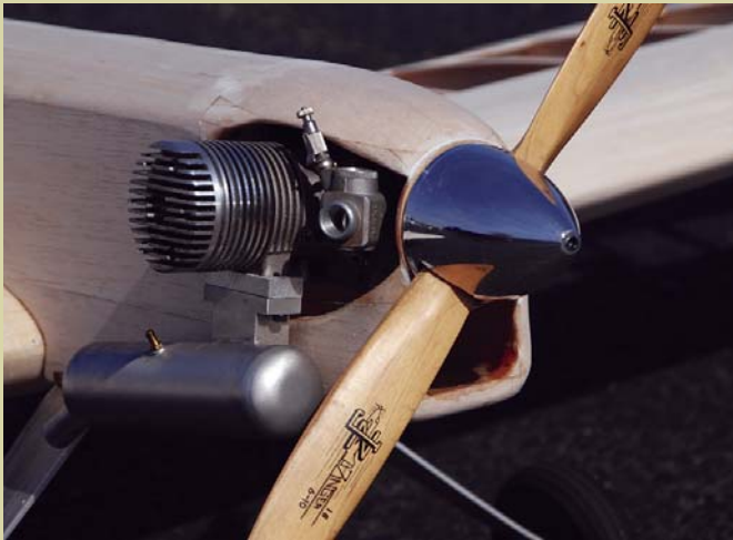
The cutout is large enough through which to pull out the Moki 1.80. It is mounted sideways, so that the standard muffer tucks in tightly against the fuselage. Balsa blocks are faired into the spinner.
