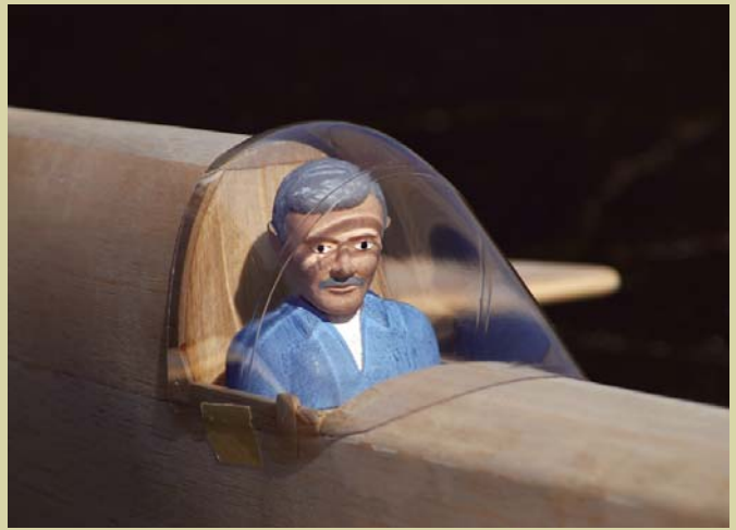
The plastic canopy was cut from a Sig Four-Star 120. A Williams Brothers plastic pilot is finished in honor of the project creator. Small screws hold these parts in place.
