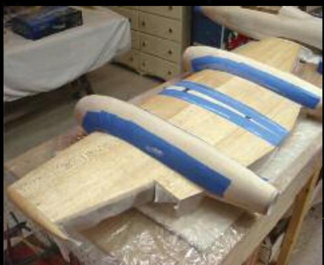
**Top:** The canopy plug was built-up from balsa and plywood. The plug was glassed, primed, and sanded before casting a permanent plug to form the canopy cover.
