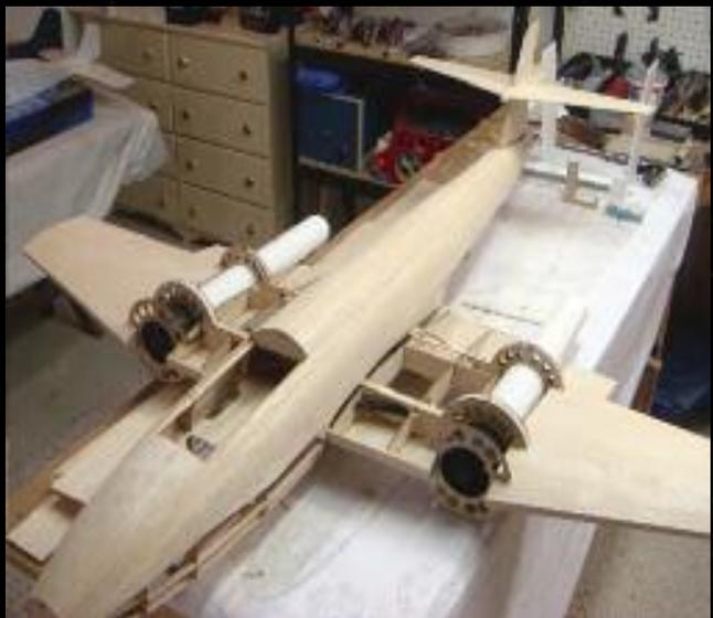
Glue R1 through R5 in the proper positions on the main spar. Glue the landing gear plates and R3C in place. Glue the rear spar assembly into position with RS2 up. Glue triangle stock around the landing gear plates and R1. Glue vertical grain balsa blocks to the rear of the rear spar for the wing mounting bolts.
