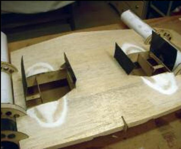
**Left:** The composite gear doors are cut and trimmed to fit. Control surface hinges were used to hinge them in place. An over-center spring holds the inner door open and closed. A wheel hits a lever to trip it.
