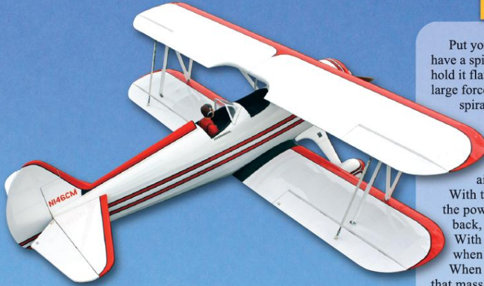
The big IMAA-legal Great Planes Super Stearman sometimes made fine takeoffs but could be difficult to keep on the runway with a side wind. The JR G770 3D Gyro gave it a totally different personality on takeoff.
