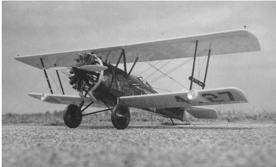
Pitcairn Mailwing – Had a 39" wingspan and was powered by a McCoy 35. Bill Winter called it a Control Line masterpiece when he published it in American Aircraft Modeler . An excellent performer, it placed third in 1968 Nationals at Olathe, Kansas.
