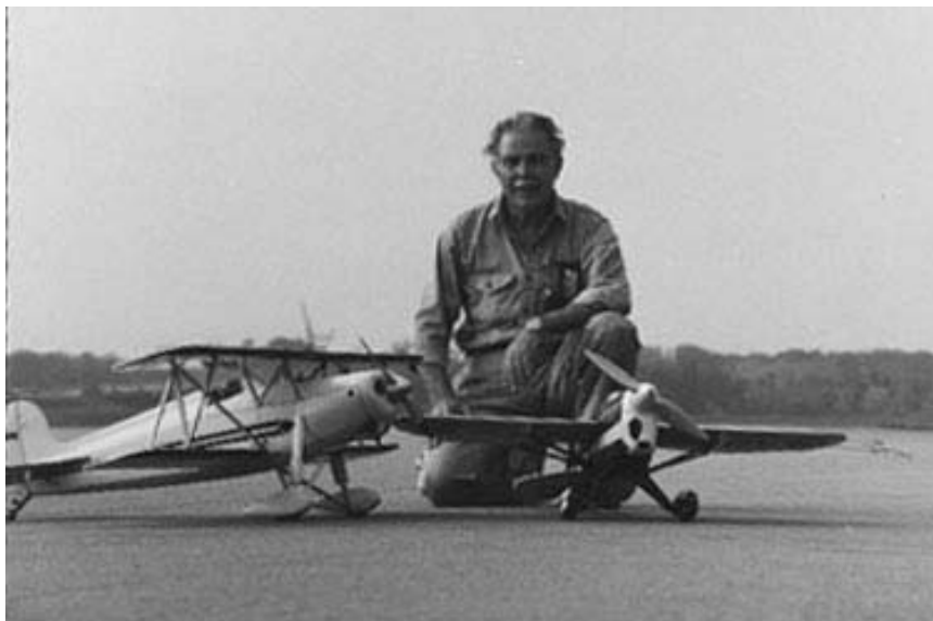
Borg Parakeet and Art Chester Special. Richard Borg, who modified a Rose Parakeet design, furnished dozens of photos and drawings to enable me to design and build a very accurate model. The model flies great with an O.S. 46 engine. It won a High Static award at the 2000 Nationals. The Art Chester Special flies great, but gets bouncy on landings. It placed third in 1999 and 2000 Nationals and was featured in Model Aviation as a construction article - and I am in the photo also.
