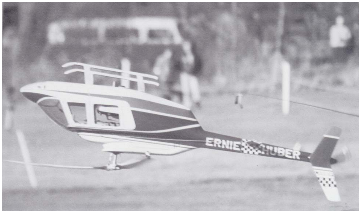
This is an actual photograph of the first inverted hover of an RC helicopter. Notice the reverse coning of the blades.
