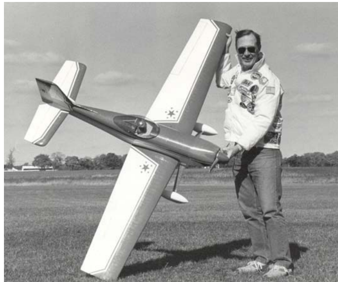
LEFT: 1984 – Dick with his Firebolt, an aerobatic design. It was a canard forward swept wing twin finned pusher aircraft that was .40-powered and had a 57-inch wingspan. This was featured in a construction model in Model Aviation magazine.
