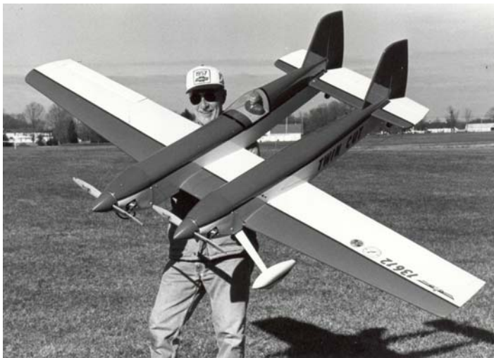
LEFT: 1998 – Dick with his Twin Cut, an aerobatic twin engine design. It had a unique layout, unequal length fuselage, gas burner engines and overlapping propellers. The 104-inch wingspan model was featured in a construction article in Model Aviation magazine.
