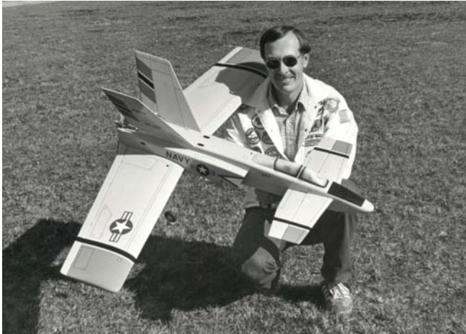
LEFT: 1984 – Dick with his Firebolt, an aerobatic design. It was a canard forward swept wing twin finned pusher aircraft that was .40-powered and had a 57-inch wingspan. This was featured in a construction model in Model Aviation magazine.
