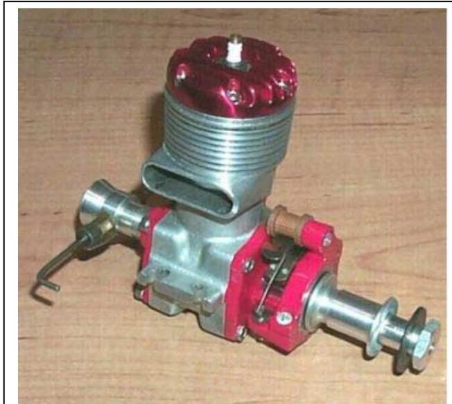
A McCoy 60 I machined and converted to ignition.
