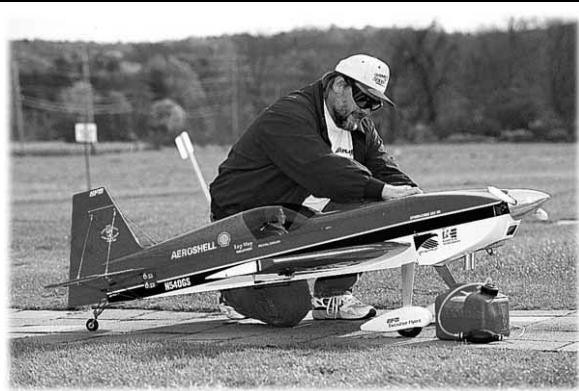
October 1999 - Me with my Giant Scale Planes GS-300 Staudacher powered by a 60cc 3W gas engine and equipped with a JR 10SX radio for control. This was my favorite plane for a long time.
