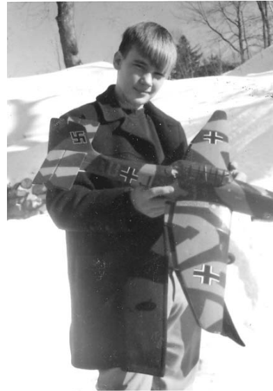
1970- A Guillows Junkers JU-87B Stuka dive-bomber, converted to U-control, sheeted with balsa and finished with AeroGloss and Sig dope. It had a Fox .09 engine and 34 \frac{1}{4} -inch wingspan.
