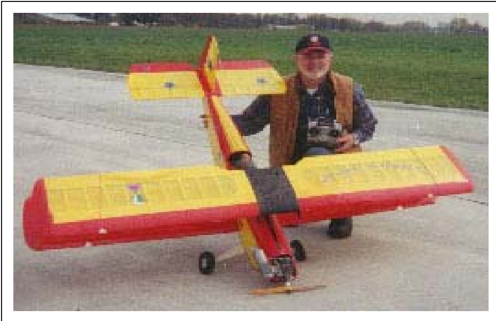
Lazy Ace Kit, built by R. Weeks in 2002. Specs: Chuck Cunningham design. 87 inch wingspan. 11 lbs, 5 oz. O.S. 91 two-stroke 13X6 prop. Monokote.
