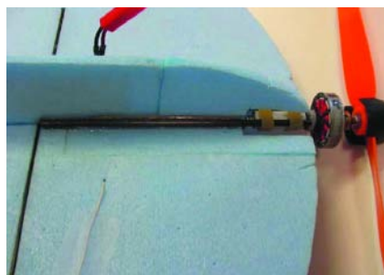
Carbon tubing in proper placement.
