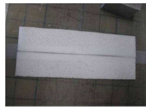
Now we run our tape the full length of the aileron. The bevel is on the bottom.
