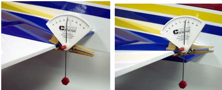
Erik and Mike used a CRC deflection gauge to ensure the desired (and equal) amount of deflection on both sides.
