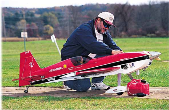
October 1999: Me with my Giant Scale Planes GS-300 Staudacher powered by a 60cc 3W gas engine and equipped with a JR 10SX radio for control. This was my favorite plane for a long time.
