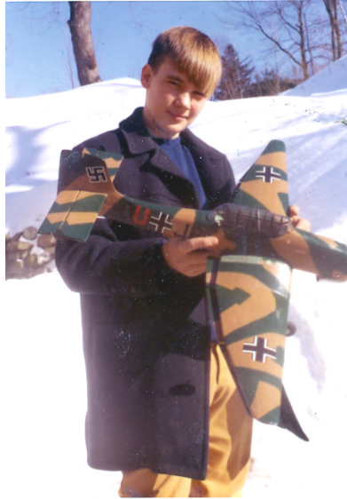
1970: A Guillow's Junkers JU-87B Stuka dive-bomber, converted to U-control, sheeted with balsa and finished with AeroGloss and Sig dope. It had a Fox .09 engine and 3¼-inch wingspan.
