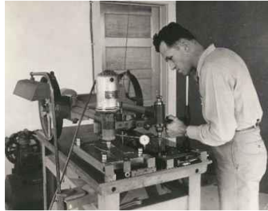
1952: Joe Stanzel produces a product on the duplicating engraving machine.
