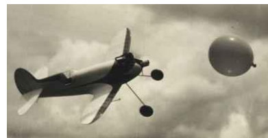
1940: The Baby Shark, a single-line, G-line Speed ship with a 24-inch wingspan.
