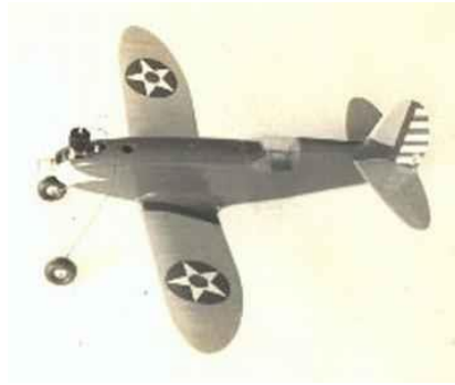
1941: The Shark P-60 Class C, a gas-powered G-line army-type pursuit airplane with a 36-inch wingspan.
