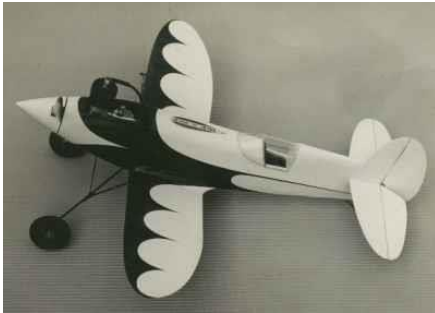
1941: The Super G Shark, a gas-powered, two-line control kit with full in-flight elevator control.
