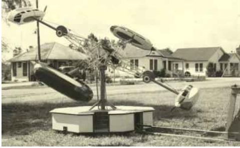
1940: The Stanzels' amusement park ride, the G-Ride, had four propeller-driven ships powered by an electric motor.
