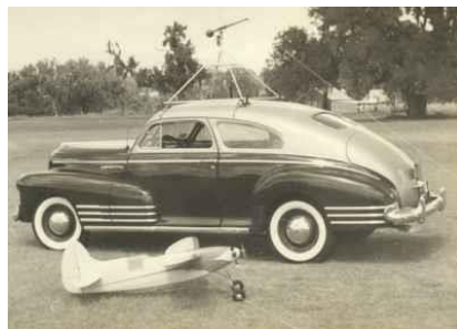
Test flying the target airplane, which was attached to a line and secured to a rotating arm mounted on the top of the vehicle.
