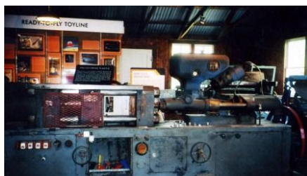
Injection molding machine from 1946, probably the first such machine in Texas.
