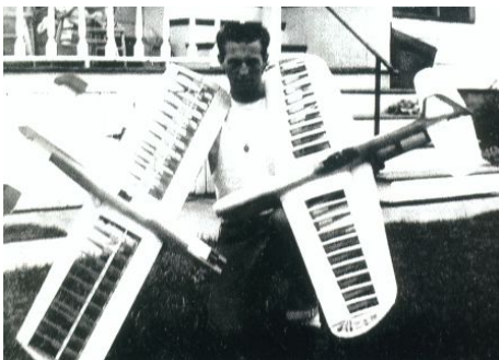
Bob Sonnleitner displays two unfinished examples of nearly five-foot wingspan aerobatic models, prior to covering and painting. It was quite a journey from the earlier 9-inch span paper-and-pine gliders to these 1/2-horsepower balsa beauties. [Sonnleitner Photo]
