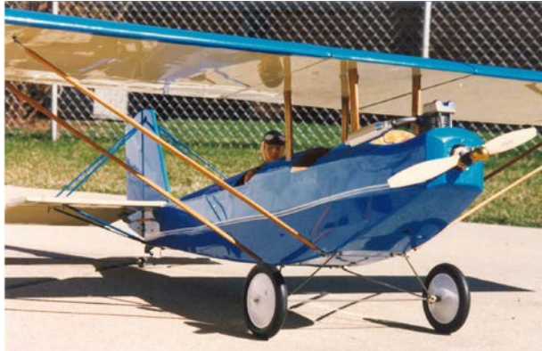
BOTH ABOVE: June 1997: Sidney's quarter-scale version of his original Pietenpol Free Flight scale model. This model is 84-inches with rudder, elevator, aileron and throttle controls. It has a .91cc four-stroke engine. Sidney added more details after these photos were taken.
