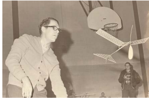
Jim Richmond's attempt sometime around 1972 or 1973 to beat the rules. Note that there are no ribs in the wing, no leading edge on the stabilizer or rudder. The model had a sheet propeller as no built-ups were allowed. This was probably the only time he placed low at 10 th .
