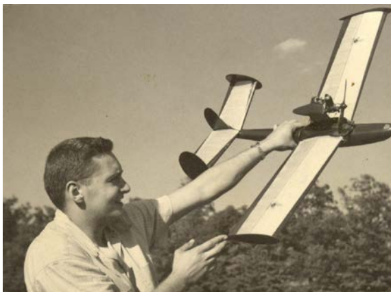
1951: Sidney at age 25, holding his original Flying Boat with an Arden .09 on glow. It was a very stable flyer with yellow silkspan and maroon paint. There were Ohlsson and Rice decals on the wing and a ballast box in the nose. This picture was taken in Van Cortland Park in Bronx, New York.
