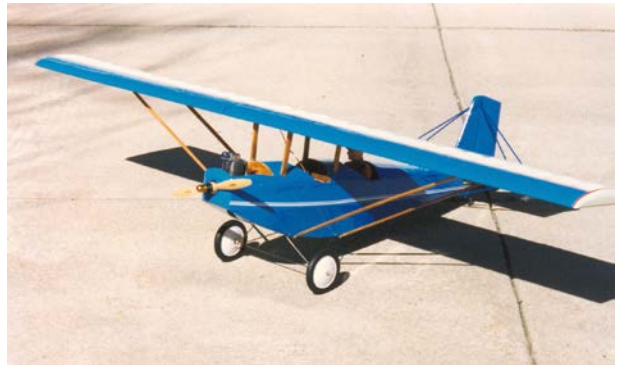
BOTH ABOVE: June 1997: Sidney's quarter-scale version of his original Pietenpol Free Flight scale model. This model is 84-inches with rudder, elevator, aileron and throttle controls. It has a .91cc four-stroke engine. Sidney added more details after these photos were taken.
