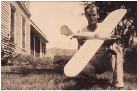
Carl at age 16 holding an early U-Control model powered by an OK Super 60 using the three-line equalized tension system.
