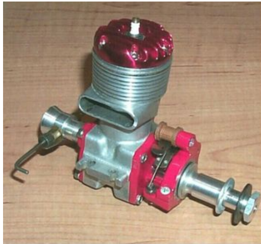
A McCoy 60 I machined and converted to ignition.
