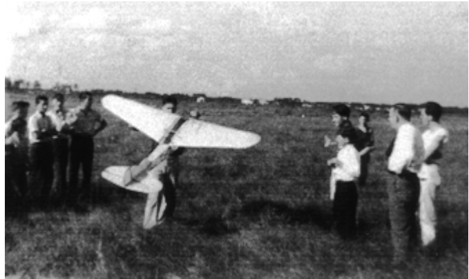
Above and left: 1938: Elmer Wasman with his second version Radio Control model called the White Peril. The four-bladed windmill-type propeller to actuate controls is located midway in the fuselage.
