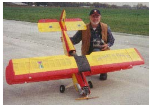
2002: Lazy Ace kit built by Roger Weeks. Specs: Chuck Cunningham design, 87-inch wingspan, 11 lbs 5 oz, O.S. 91 two-stroke 13X6 prop, covered in Monokote
