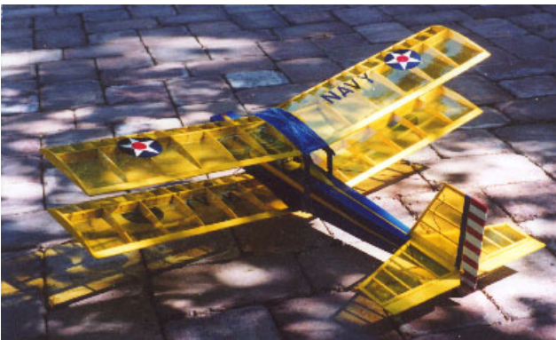
2004: Ugly Bipe, built by Roger Weeks. Specs: Laser-cut BMJR Kit, 33" wingspan, 12.05 oz, .010 Astro geared, brushless, covered in transparent Ultracoat
