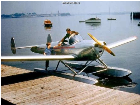
One of the two experimental Ercoupes equipped with EDO floats, showing the strut arrangement.
