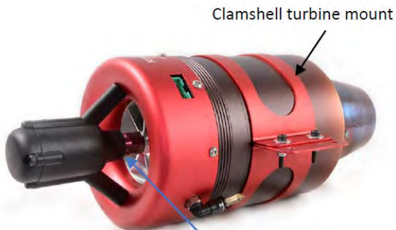
Clamshell turbine mount Starter motor O-ring sandwiched between compressor “spinner” and starter motor clutch.
