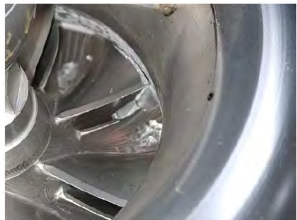
Extensive inlet and compressor damage due to front bearing failure
