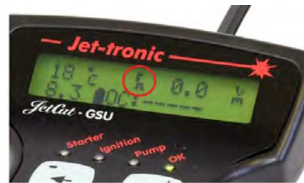
Jetcat GSU showing failsafe activated
