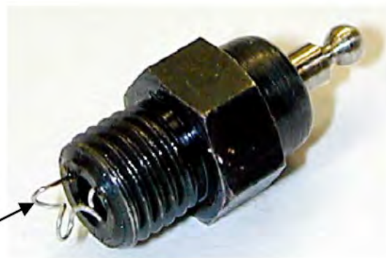
Two coils pulled clear of base and into “slipstream”.
