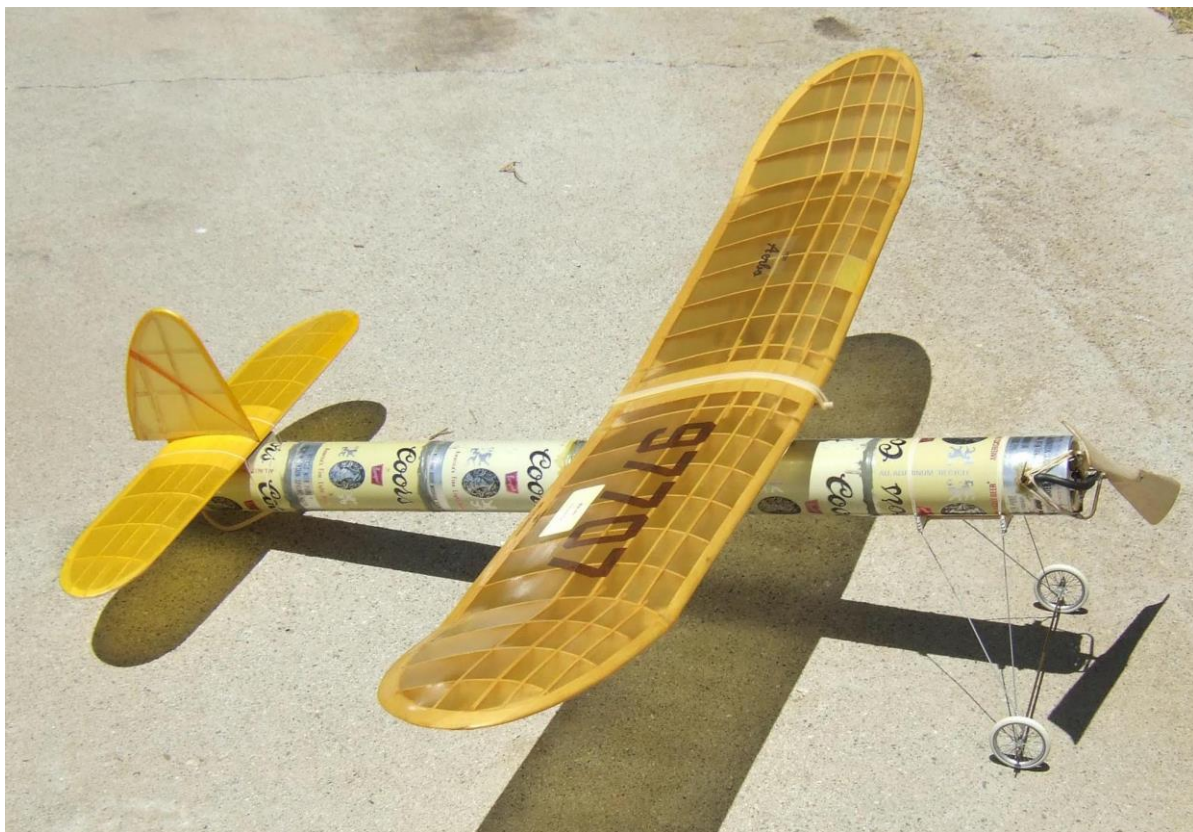
Coors can air tank on Tom Lay's compressed air model. (Source: Image provided by Bill Bickel.)
