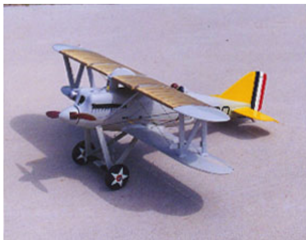
Curtiss CR-2. It has a 45" wingspan and is powered by an O.S. 61. It won in High Static and first place in the 2000 Nationals Designer Control Line Event. It was featured in a construction article in Flying Models magazine.
