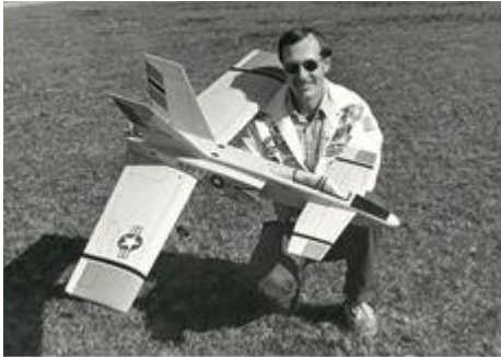
1984: Dick with his Firebolt, an aerobatic design. It was a canard forward swept wing twin finned pusher aircraft that was .40-powered and had a 57-inch wingspan. This was featured in a construction model in Model Aviation magazine.
