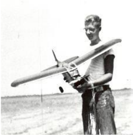
1952: Dick flying Radio Control at Hadley Airport in New Jersey with his Trixter Beam powered by a K&B .15, 27 mc single-channel radio equipment by Control Master.
