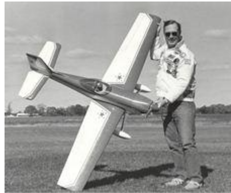
1989: Dick with one of the earliest larger model aircraft designs for the newly popular "chainsaw" gas engines. This is his Prime Cut, fully aerobatic model. It was featured in a construction article in Model Aviation magazine and then commercially kitted. The model had a 90-inch wingspan.
