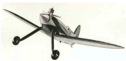
1939: The Tiger Shark, fully built. It was a gas-powered, single Control G-line model. Stanzel had a control-for-miniature-airplane patent.
