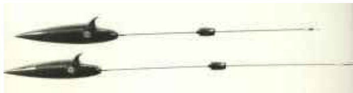
1945: Monoline control handles with sliding control knobs, which applied torque to the line.
