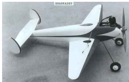
1947: The Sharkadet, a gas-powered G-liner designed for the new Control-It and Thum-it devices.
