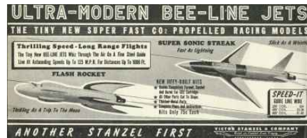
1947: Bee-Line Jets were marketed in kit form as the Flash Rocket and Super Sonic Streak, propelled along a steel line by a CO 2 gas cartridge.
