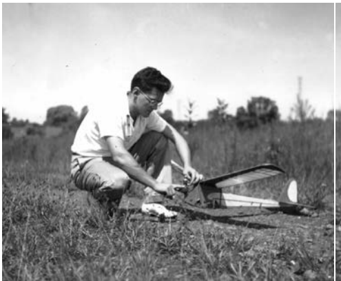
Frank cranking up a one-of-a-kind Tlush engine, a 1/2-in. bore, 5/8 stroke engine. The airplane was named Mite and was featured in a 1937 issue of Air Trails magazine.
