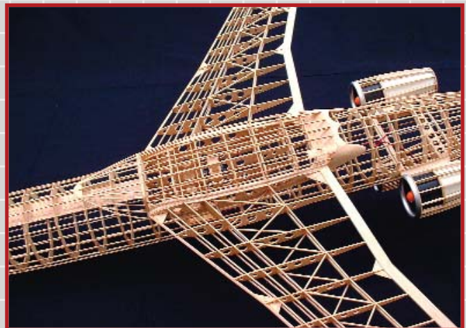
Since the center wing section is built with the fuselage, the correct fit is guaranteed. Be sure to select hard balsa for the stringers; they will add the needed strength.
