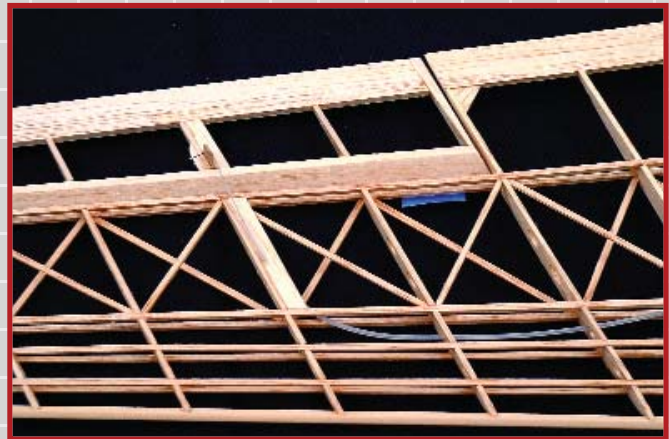
PTFE spaghetti tubing is used to house the 0.015-inch music wire inside the 0.034-inch ID tube and actuate the top hinged aileron controls.
