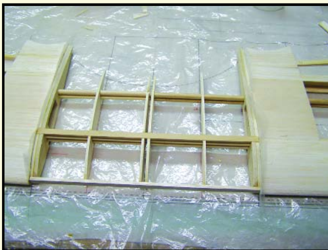
The center-section of the upper wing secures the dowel-rod wing joiners inside plywood ribs. The completed sheeting is sanded flush with the outer panels.
