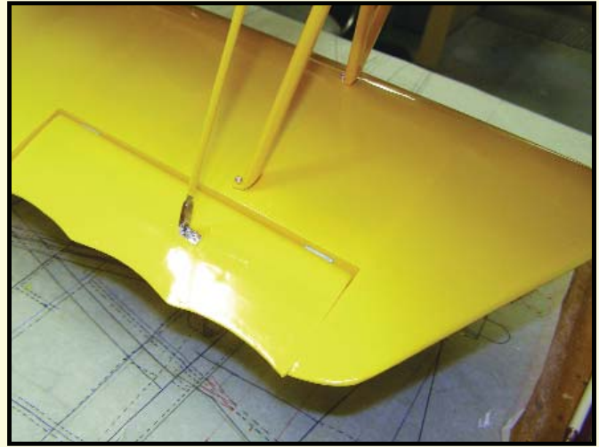
Pushrods from upper to lower aileron are linked to aluminum angle brackets located in hard points near the LE of the control surface.
