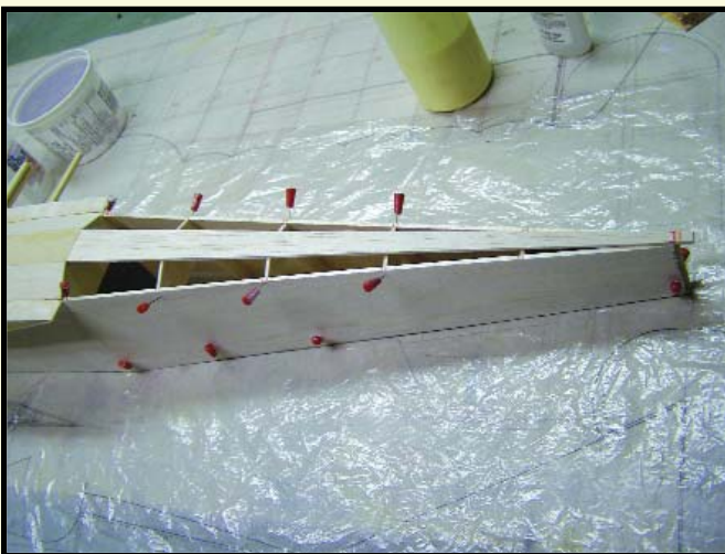
Once the fuselage sides are pulled together, the lower sheeting and longerons can be added. Watch out for twisting and keep the tail post square.
