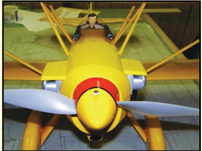
The simulated engine is made from scrap balsa that is covered and painted to match the IO-235 four-cylinder engine used in the full-scale aircraft.
