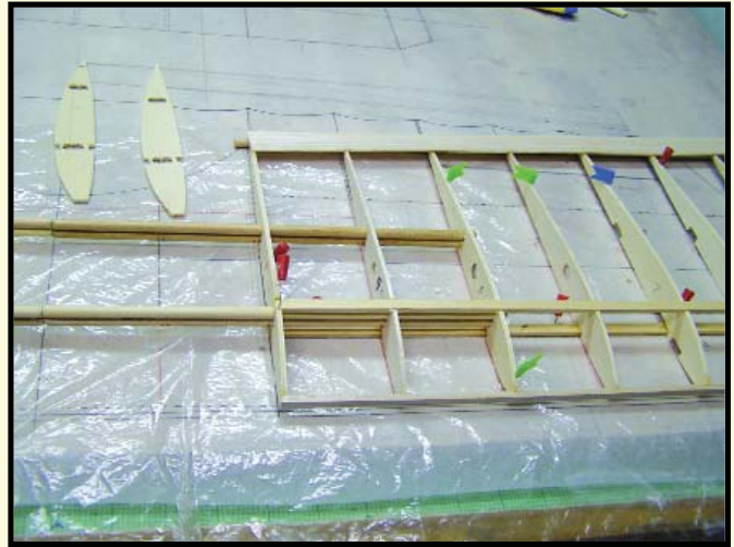
Wing panels join the center-sections with stacked dowel rods at the apex of the rib shape. Center-area ribs are made from light plywood.
