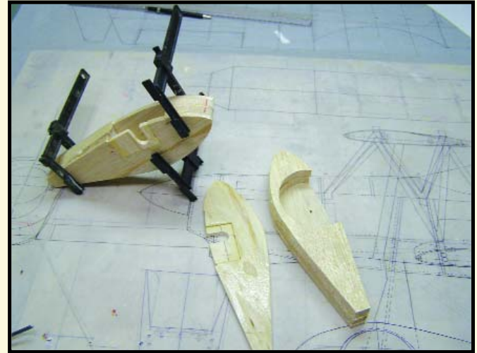
The wooden sections of the wheel pants are laminated with wood glue, which is easy to sand later. Plywood buried inside acts as a mounting point.
