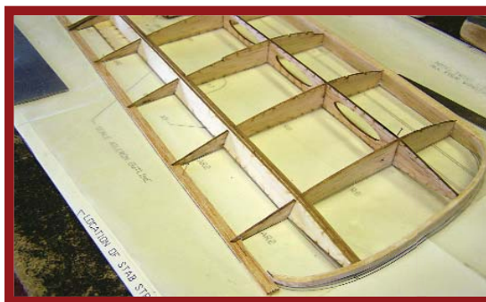
Aileron ribs and front hinge spars are adhered in place directly on the wing assembly while the wing is still pinned to the building board.
