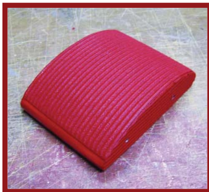
The top-wing center-section is covered with corrugated foam from Titanic Airlines, sanded to shape, and painted with Model Master Acryl.
