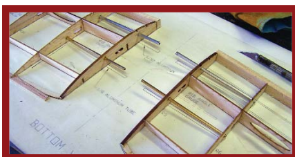
The 5/32-inch-OD and 1/8-inch-OD rear aluminum wing-attachment tubes are glued in place on the bottom wing assemblies.
