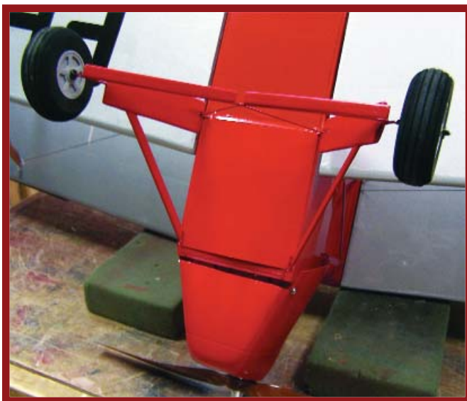
Battery access is through a plastic hatch on the fuselage bottom. Motor cooling air exits the gap at the bottom of the cowl at the firewall.
