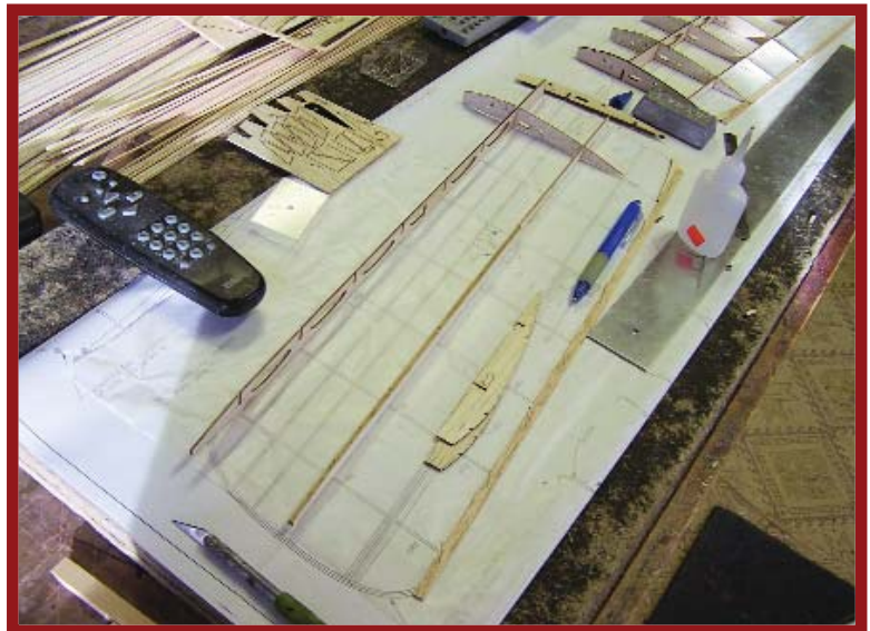
The wing assembly begins with all spars, ribs, and TEs glued together over the plans. Once the basic right wing is framed, the left wing is assembled to the same point.
