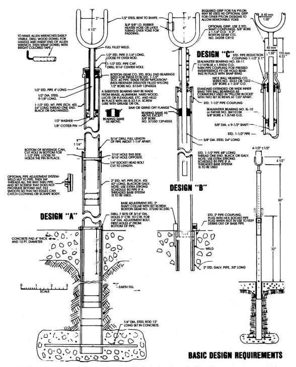
Pylon fabrication methods are optional. However, it is recommended that the design be capable of the minimum and maximum yoke heights shown and that the fork be within the limitations given. The pylon shall be capable of withstanding a 150-pound horizontal pull on the yoke when it is at the maximum height position.
