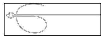
1) Run at least six inches of line through the eye of the clip, and fold to make two parallel lines. Bring the tag end of the line back in a circle toward the clip.
